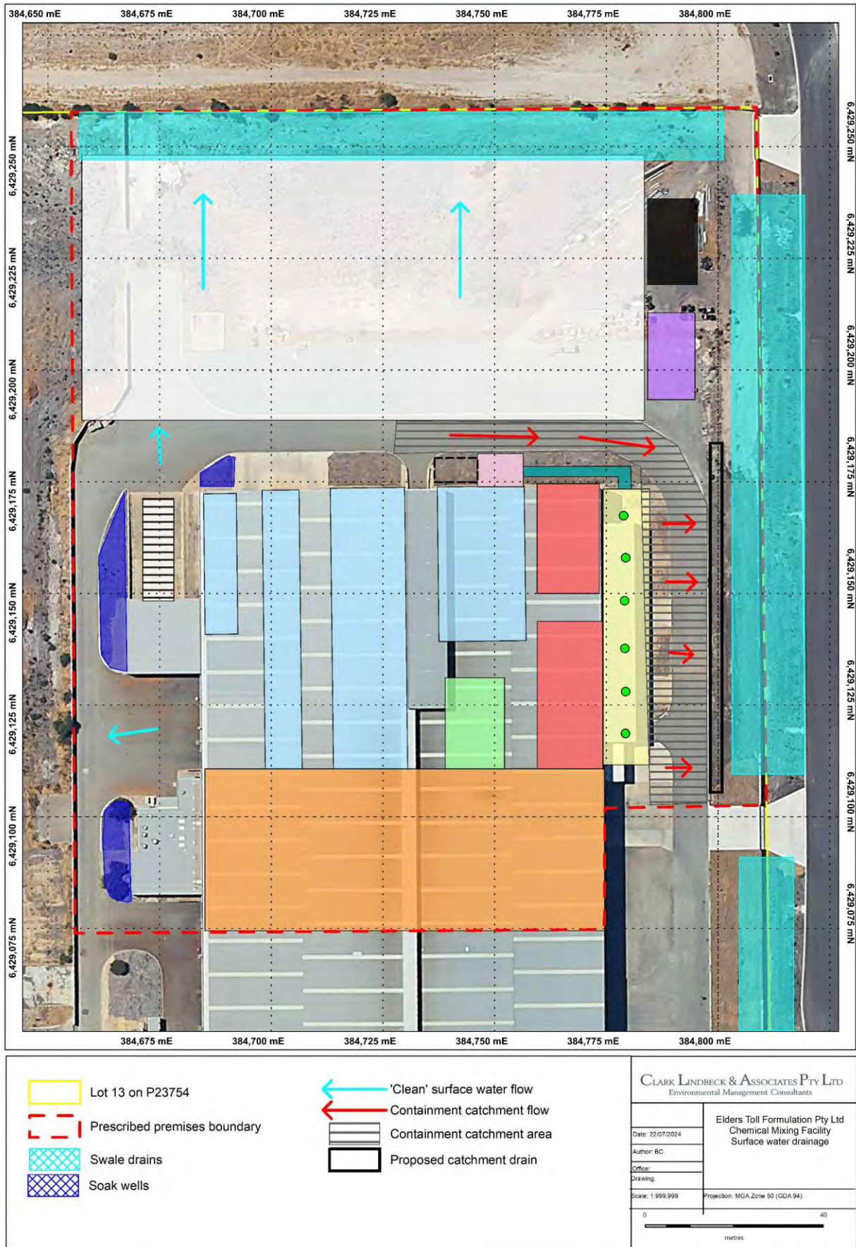
Figure 5: Surface water flow/containment outside of the existing building
