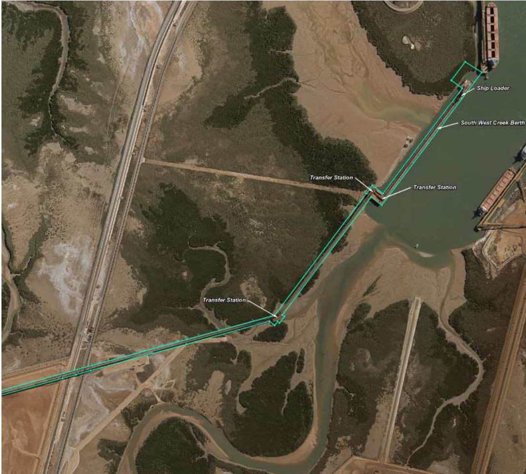
Figure 3: Overland conveyor and ship loading area layout
