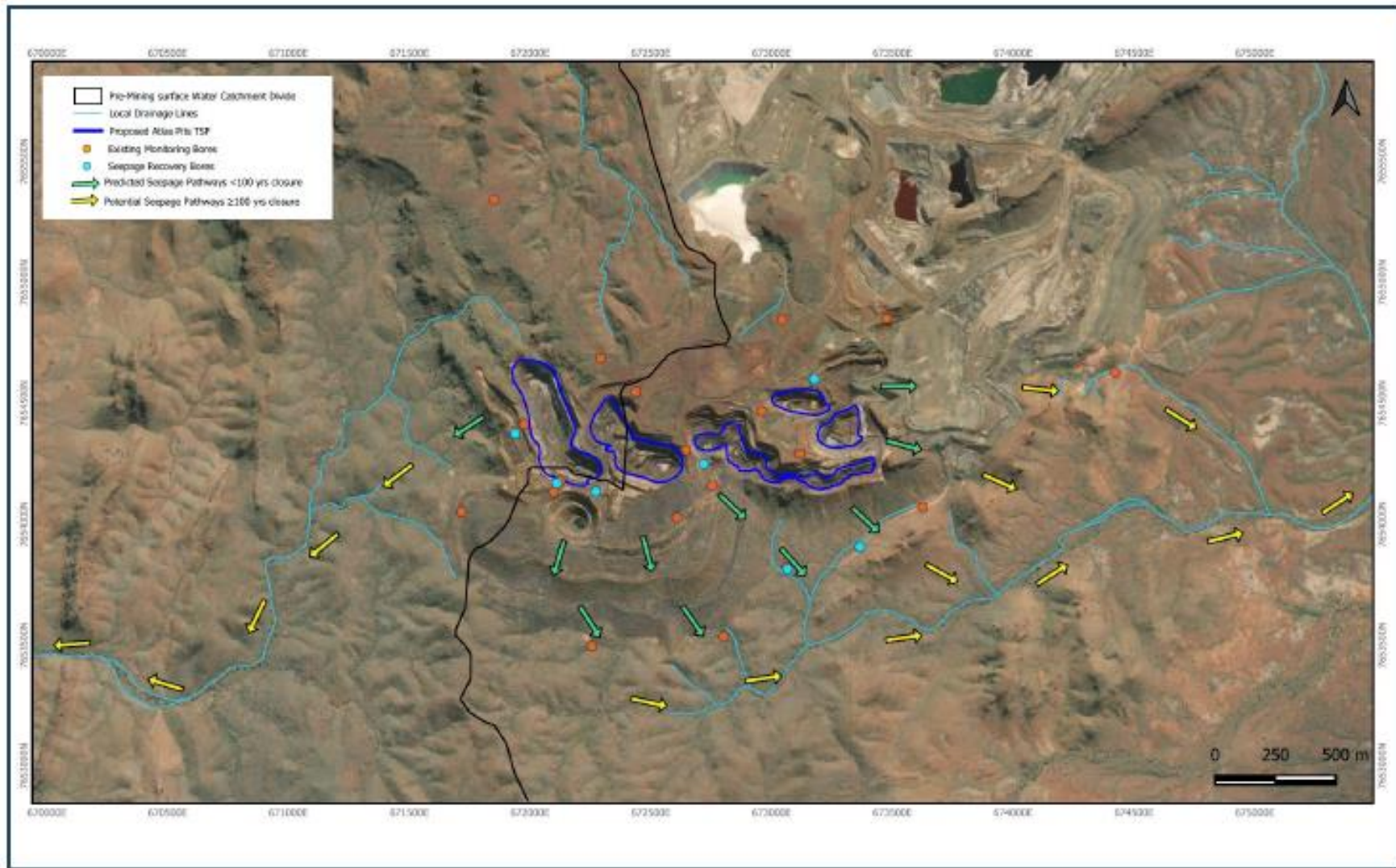
Figure 5 – Modelled surface pathway of groundwater seepage (without controls) and location of existing and proposed bores.
